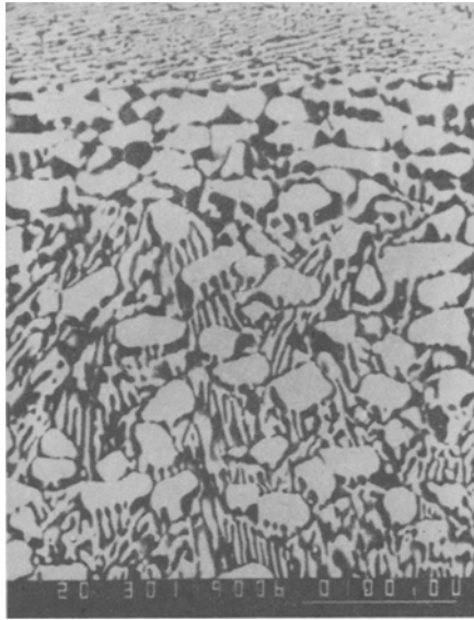
Fig. 3 The beginning of the interfacial layer remelted in conditions of microgravity; direction of solidification: from the left to the right; the part of ingot \text{PbCl}_2\text{-AgCl} solidified under terrestrial conditions is on the left side; \text{PbCl}_2 phase is white, \text{AgCl} phase is black (backscattered electron image, magn. 300\times , white abscissa on the right = 100\ \mu\text{m} )
